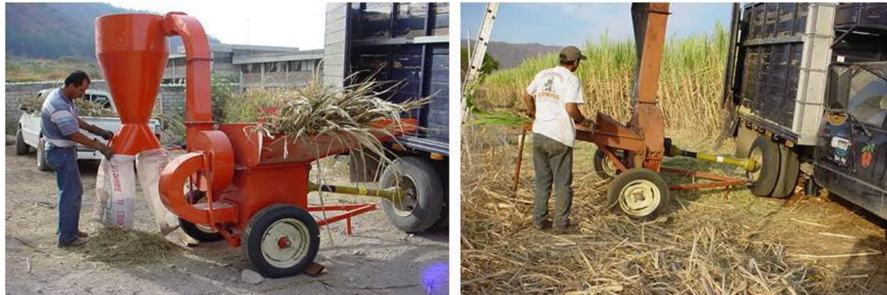
Figure 2. Fixed agricultural equipment connected to the truck's power take-off
